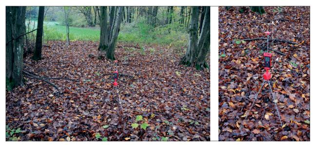
Fig. 1: DistoX on the calibration tool in the field work location. The coordinate system is defined as in Heeb (2009) (Photo: M. Perne).
