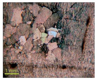
Fig. 12:  $II^{nd}$  phase of A-C transformation (optical microscope); calcite crystals with neater boundaries lack the intercrystalline voids.
