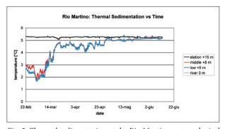
Fig. 5: Thermal sedimentation at the Rio Martino meteorological station. It is possible to see a seasonal dependence of its structure, that it tends to disappear during summer.
