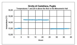
Fig. 4: Thermal sedimentation measured in the Sala Monumenti, in the Grotta di Castellana, Puglia, Italy. **The thermometer was** held for 5 hours near a monitoring station, on the floor, then moved to the upper part in the hall, then moved again to the previous position.
