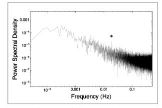
Fig. 15: Corchia cave complex (Tuscany), Eolo entrance. A typical air flow spectral power. The intrinsic harmonics are usually submerged by a pink noise.
