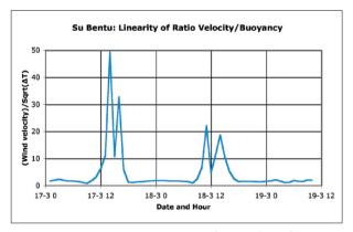
Fig. 11: Su Bentu cave, near Nuoro, Sardinia, Italy. In the convective model of air circulation, the wind velocity and the square root of the difference between internal and external temperature are proportional, then plotting one vs. the other would give a straight line. It looks far to be true.
