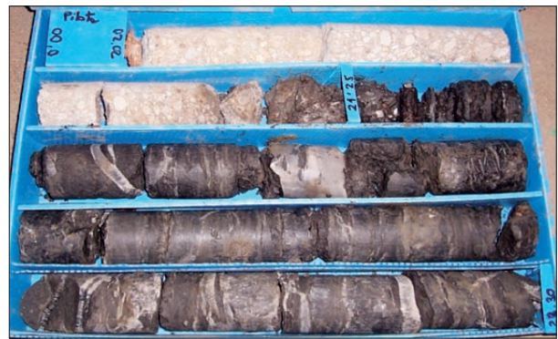
Fig. 15: Inspection samples of the endpoints of 1,000 mm diameter piles which confirm the presence of folded gypsum without signs of karstification.
