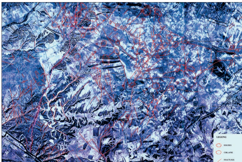
Fig. 2: Layout of the fracture network, areas with dolines and collapses in south-eastern Madrid.
