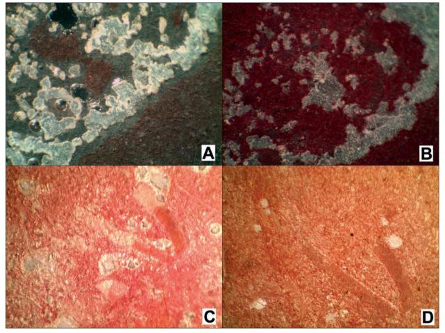
*Fig. 2: Microphotographs of a tablet surface, stained acetate peels. Red, purple = calcite; pink, white = dolomite. A and C – before, B and D - after the field (subsoil) exposure. Note the dissolution effects (B) and complete removal (D) of dolomite grains.*
