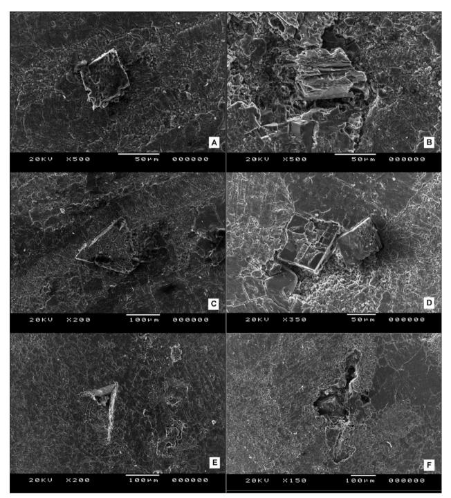
*Fig. 3: SEM images of the-limestone tablets surface; A) idiomorphic dolomite grain in calcite matrix; B) cavities along a dolomite grain; C) hypidiomorphic dolomite grain in calcite matrix; D) cavities on contacts between calcite matrix and dolomite grain; E) mold/cavity left by removal of a dolomite grain; F) void in a limestone tablet, dolomite crystal barely visible in the cavity.*
