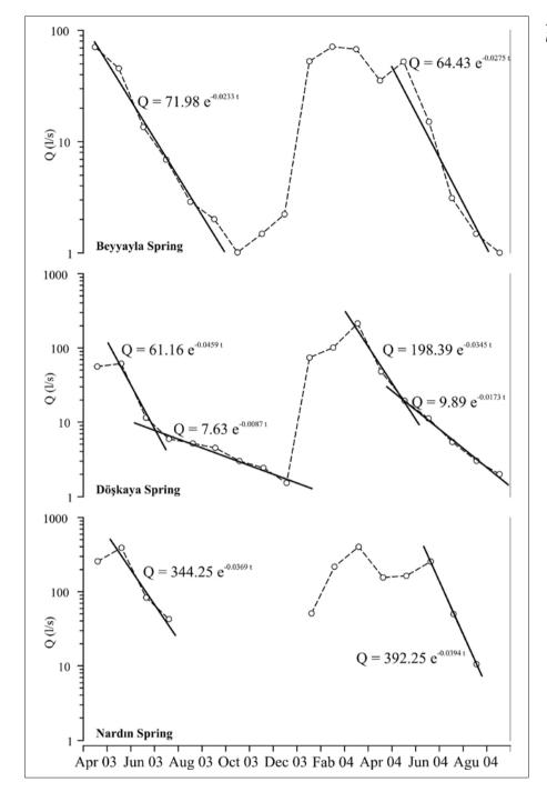
Fig. 6: Recession curve of Beyyayla, Döşkaya and Nardın spring.
