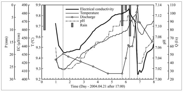
Fig. 5: Chemograph for Döşkaya Spring, April 2004 storm.
