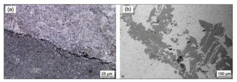
*Fig. 2: (a) Micritic limestone with stylolithe in sample DG1. Transmission light, parallel polars. (b) Dolomitized areas in calcitic veins of the limestone in sample DG1. SEM-BSE.*
