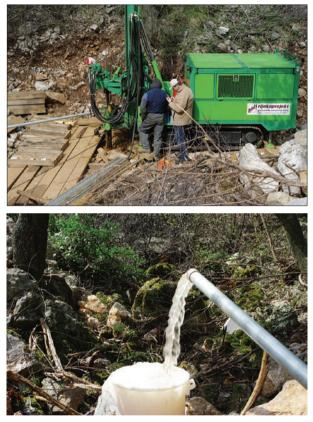
*Fig.* 13: *Pumping test of the exploration well at the location of occasional spring Sušica (Photo: R. Biondić).*
