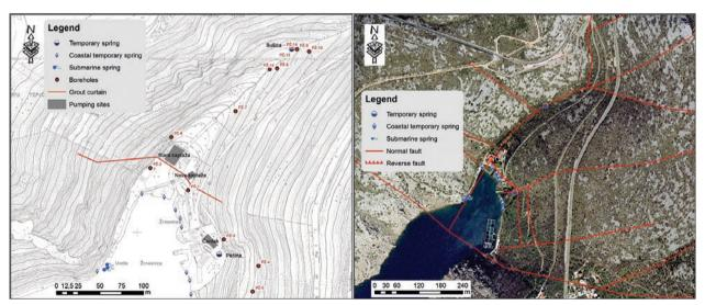
Fig. 4: Positions of the spring zone, grouting curtain, exploration boreholes, and main faults.
