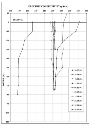
Fig. 11: Changes of electrical conductivity in the borehole PŽ-8.
