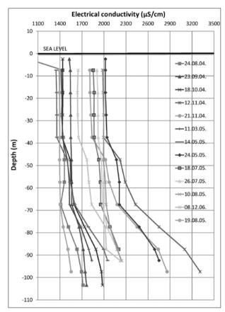
Fig. 9: Changes of electrical conductivity in the borehole PŽ-2.
