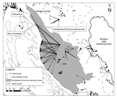
*Fig. 3: The catchment of the spring zone Novljanska Žrnovnica and tracing test from the catchment (according to Biondić, B. et al. 2007b).*
