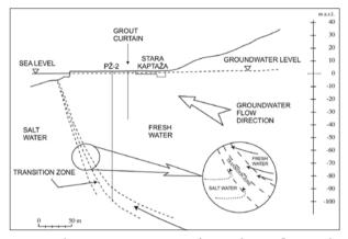
Fig. 8: Schematic representation of groundwater flow in the coastal aquifer Novljanska Žrnovnica (Biondić, B. & Biondić, R. 2003).
