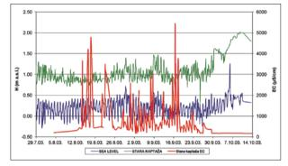
Fig. 5: Water level fluctuations, sea levels and electrical conductivity at spring Stara Kaptaža, during summer dry period 2003 (Biondić, B. et al. 2007a).
