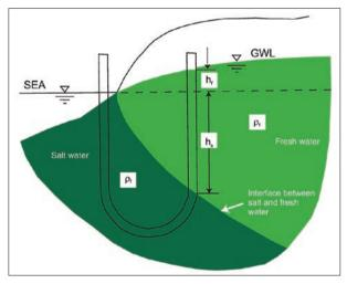
Fig. 7: Freshwater-saltwater interface according to Ghyben-Herzberg law (according to Bear & Verruijt 1994).
