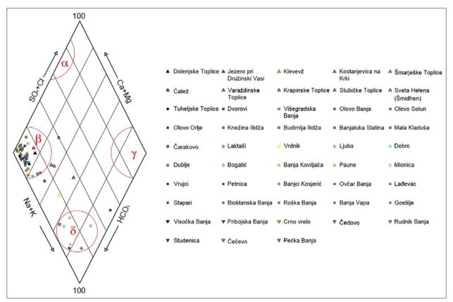
Fig. 7: Graphical survey of D'Amore- water types in the example of karst thermomineral waters of Inner Dinarides.
