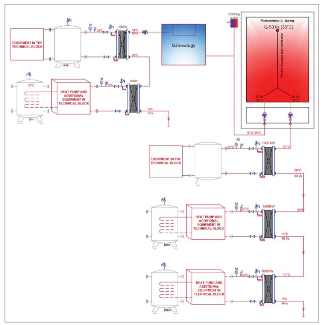
Fig. 10: Schematic survey system for multi-purpose utilisation of thermomineral waters in Pribojska Banja Spa (Milenić 2010).
