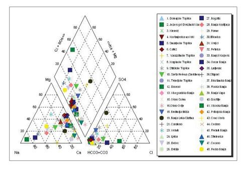
Fig. 4: Piper trilinear diagram of karst thermomineral waters of Inner Dinarides.
