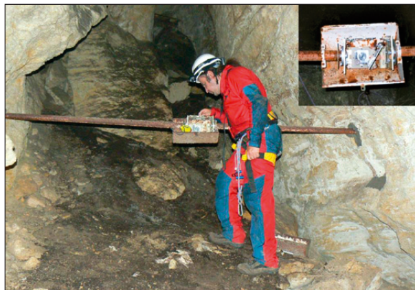
Fig. 7: Regular measurements at Golyamata Tsepnatina Cave, monitoring site M9 with monitoring gauge damaged after August 1999 Izmit Earthquake (upper right corner) (modified after Shanov & Kostov (2015)).
