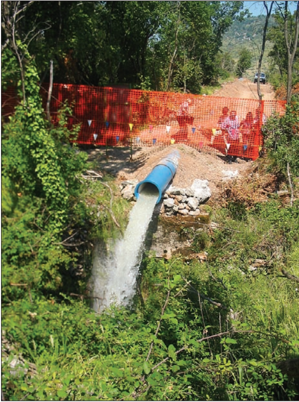
Fig. 4: Pumped groundwater from well B-10/06 discharged through a temporary pipeline (Photo: J. Urbanc).
