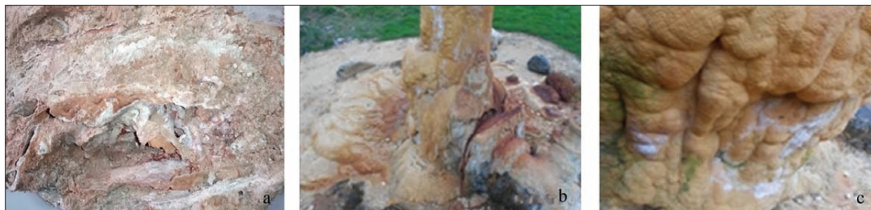
Fig. 12: Encrustation sampling points: a) well BB-1, b) well LB-4, c) well LB-5 (Photo: M. Lazić, 2014-2016).
