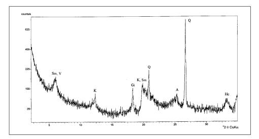
Fig. 5: A part of the X-ray diffraction pattern of the natural untreated sample of red clay No. C95B before separation, representing the mineral composition of red clay (for abbreviations see Table 3).
