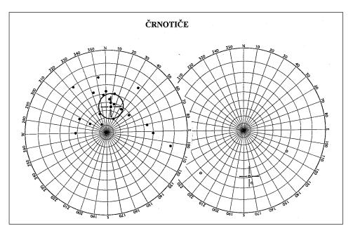
Fig. 9: Samples with normal (left side) and reverse (right side) of palaeomagnetic polarity. Stereographic projection, full (open) circles represent projection onto lower (upper) hemisphere. The mean direction calculated according to Fisher (1953) is denoted by a crossed circle, the confidence circle at the 95% probability level is circumscribed about the mean direction.
