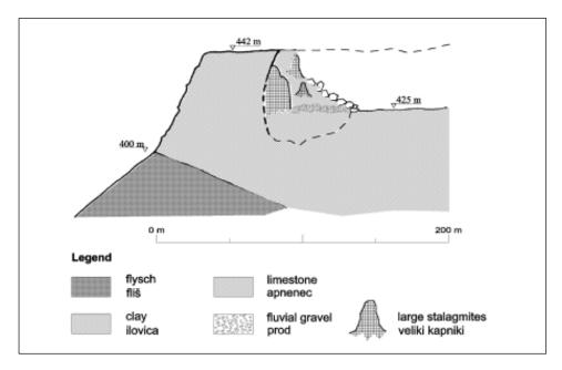
Fig. 3: Schematic cross-section of the edge of the karst plateau, quarry and studied cave.
