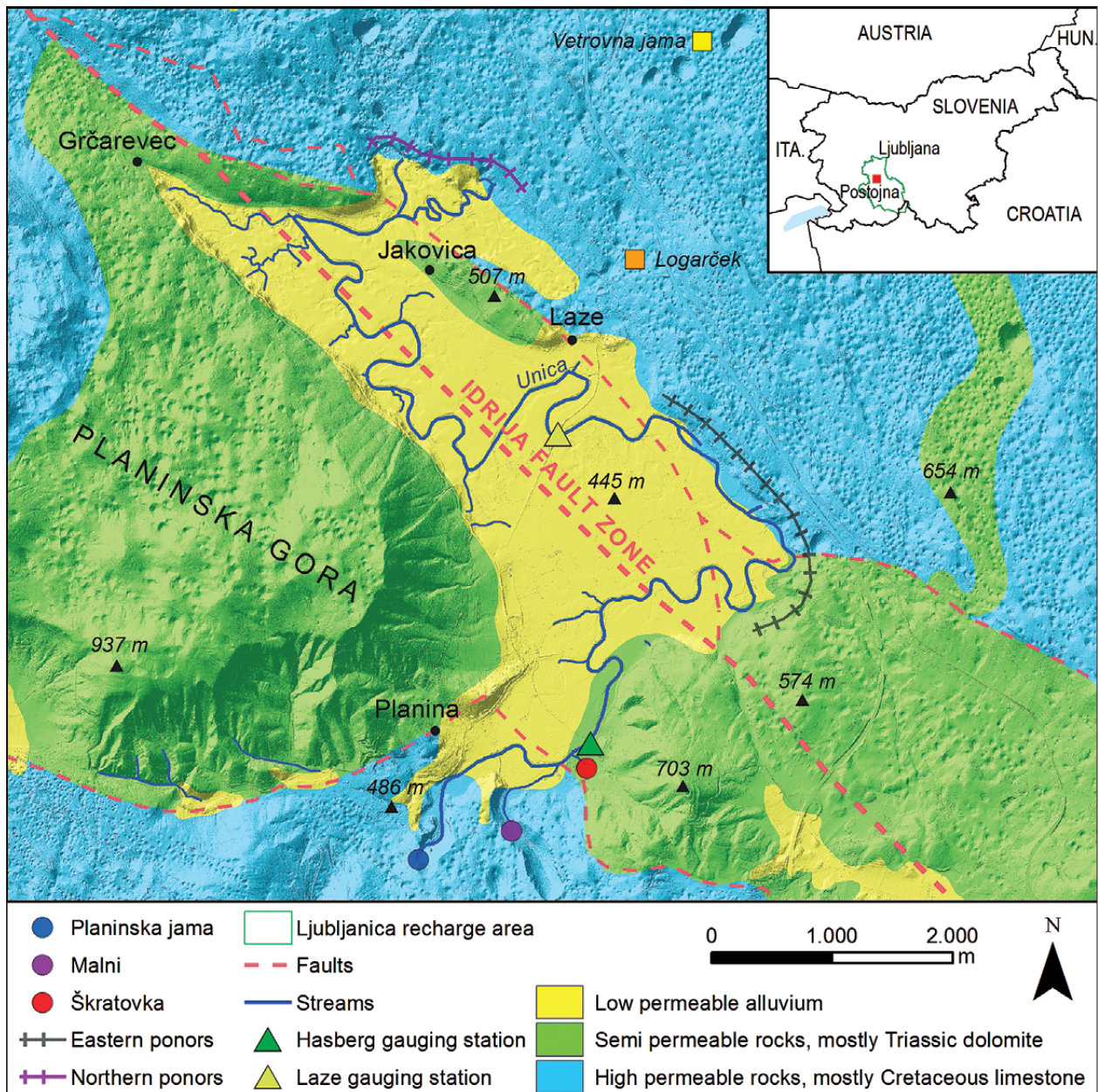
Fig. 1: Planinsko Polje and the surrounding area with the position of caves, springs, ponor areas, gauging stations and main hydrogeological units (modified after Krivic et al. (1976), DEM data from ARSO (2017b)). The upper right insert shows the regional position of the area (red square), where the Ljubljana recharge area is enclosed by the green line.
