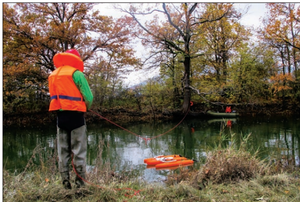
Fig. 4: Trimaran with Doppler radar dragged across the Unica River (Photo: F. Gabrovšek).
