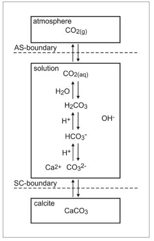
Fig. 1: Box model of basic interactions in carbonate karst.
