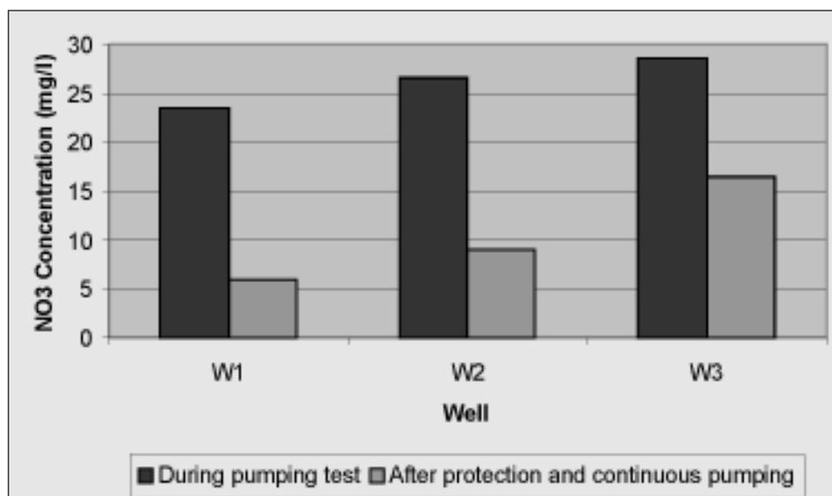
*Fig. 9: The concentration of  $\text{NO}_2$  in water samples during pumping test and after protection and continuous pumping.*
