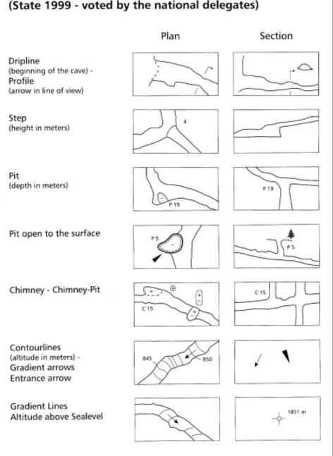
Cross-section: Cross-sections are of major importance for the understanding of a passage. For each map passage cross-sections must be drawn. The arrows indicating the direction of view are done differently, a clear indication is, however, necessary.
