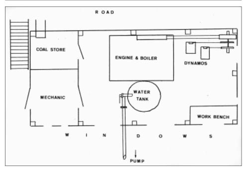
Fig. 2: The electric generating equipment outside the entrance in 1884, redrawn from a plan in the archives of Postojnska jama.
