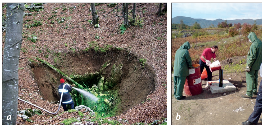
Fig. 8: Places of tracer injections – (a) in the sinkhole near the village Rastovača; (b) in the piezometric well near the village Drežnik Grad.
