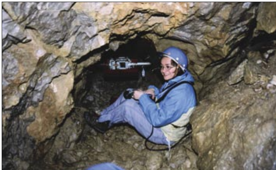
Figure 7: Artificial tunnel in Postojnska Jama and TM 71 (photo S. Šebela).
