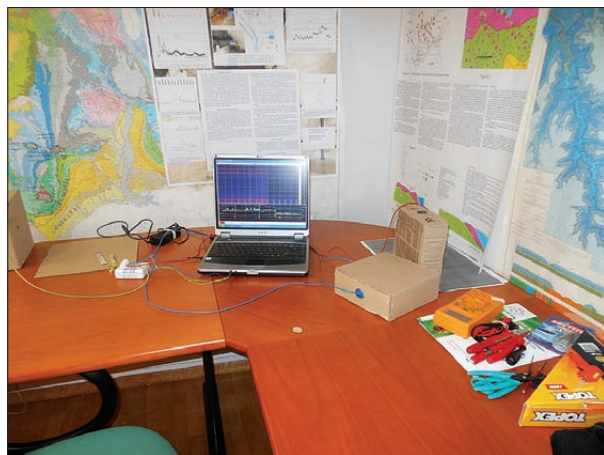
Fig. 2: Testing of the VLF receiver in office before installation in the cave (Photo: S. Šebela).
