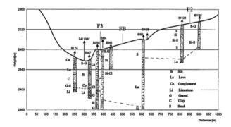
Fig. 3: Geological log of boreholes in direct to dam axis in Fig.1b, With the important F3, FB faults and F2 fault that distingushed by displacement Formatio in boreholes.
