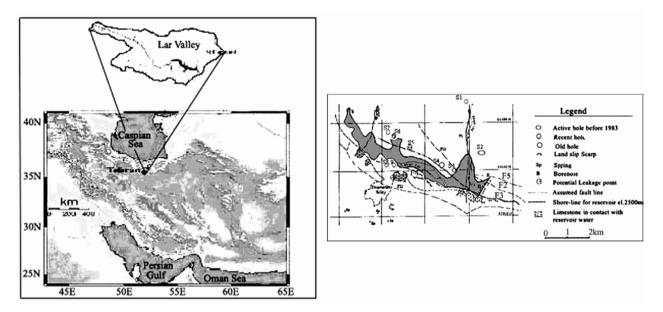
Fig.1: a) Location of the Lar dam region, northeast of Tehran. b) Location of the Lar dam and distribution of sinkholes and active faults.
