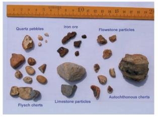
Fig. 12: Rock particles and pebbles found in the sediment.
