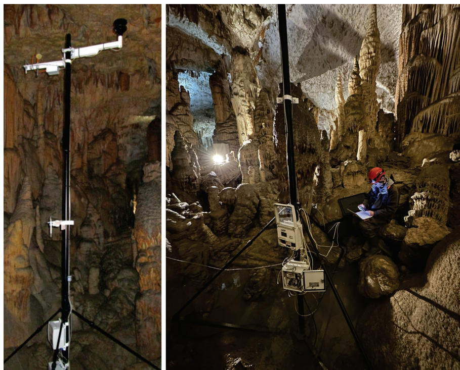
Figure 3: Diagram and constituents of automatic micrometeorological station with temperature, CO 2 and airflow probes, AMS data-logger, and storage/data processing unit.
