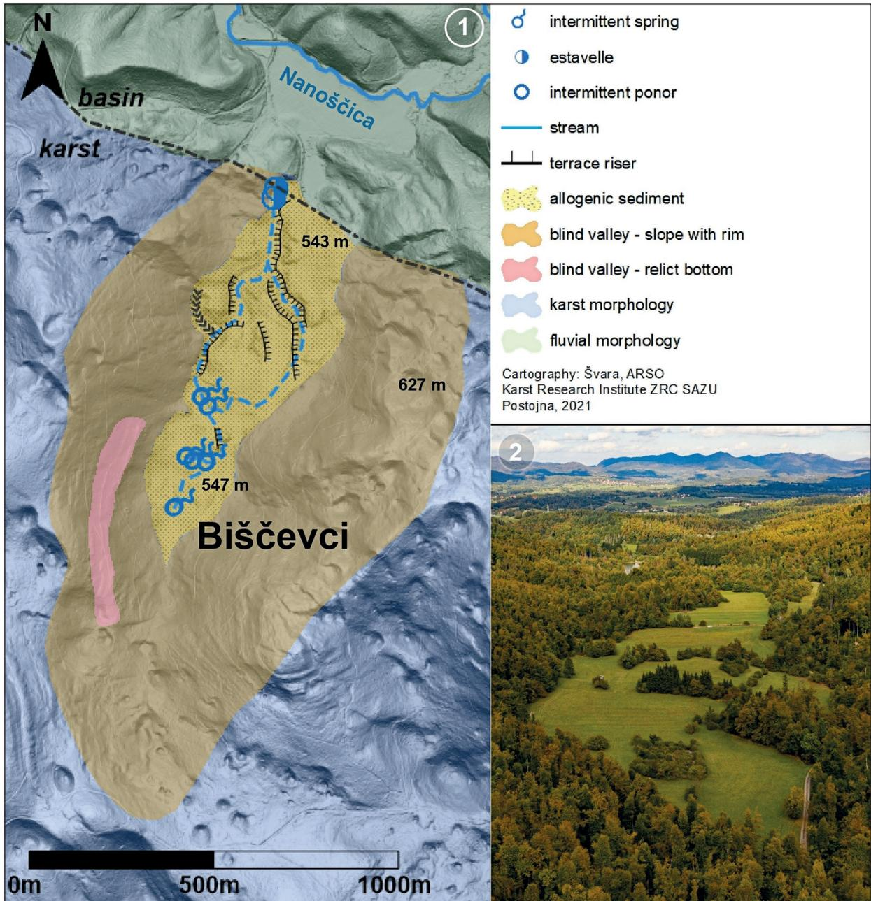
Figure 9: Geomorphological map of the Biščevci blind valley (DEM – LiDAR data, ARSO, 2021b) (1), Biščevci blind valley towards the north in dry season (2; RI-SI EPOS drone).
