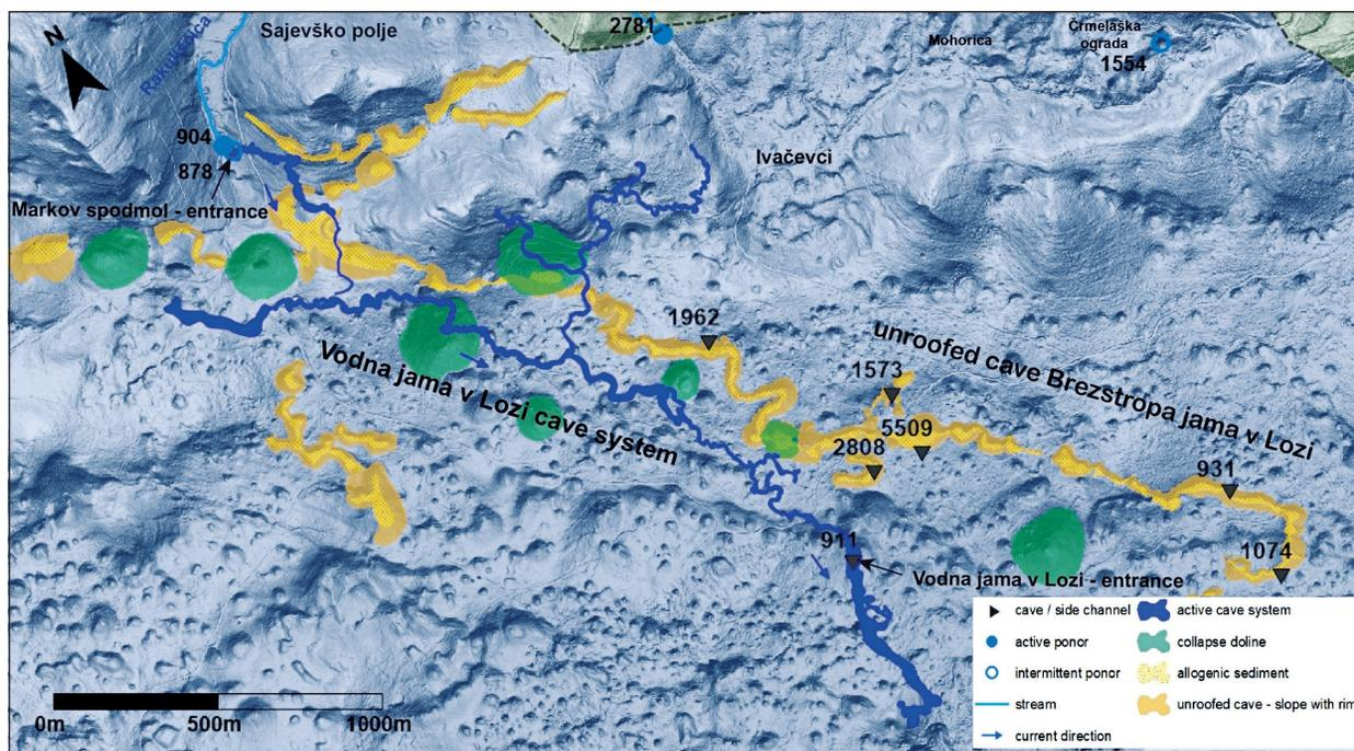
Figure 5: Location and geomorphological map of the cave system in Slavinski ravnik: active caves Markov spodmol and Vodna jama v Lozi and the unroofed cave Brezstropa jama v Lozi (DEM – LiDAR data, Geodetic department ARSO, 2021b).
