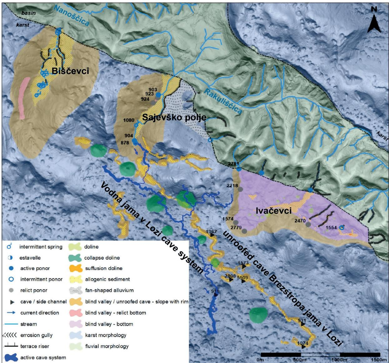
Figure 3: Geomorphological map of the study area with the locations of the cave entrances and the passages of the active and unroofed caves. (DEM - LiDAR data, ARSO, 2021b).
