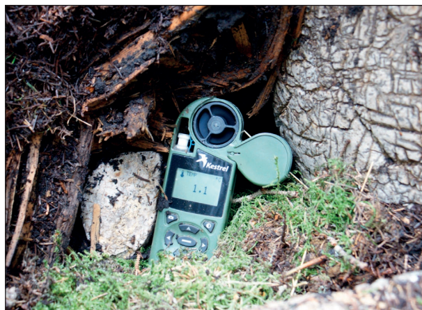
Figure 5: Measurement of airflow velocity in dwarf pine site in the southern depression (point JK).
