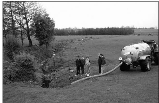
Fig. 3: Injection in a small swallow hole with the aid of an artificial injection of water (Photo: R. Meehan).
