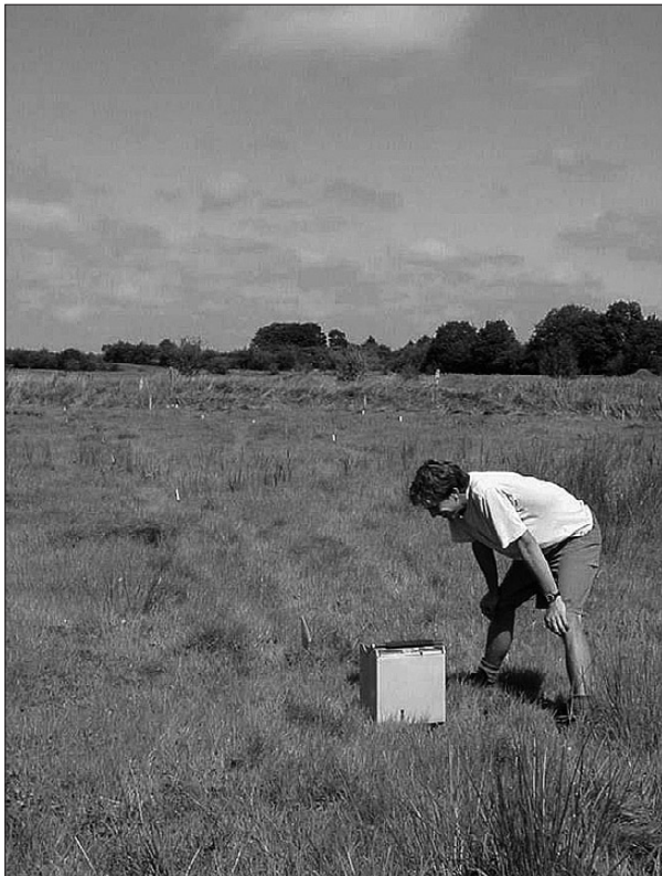
Fig. 4: Microgravity surveying being conducted at 5 m intervals in a grid system (marked out by coloured flags) (Photo: C. Hickey).
