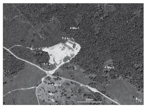
*Fig. 3: The Mozelj landfill with the two injection points (T1 and T2) and the monitoring boreholes (Mo-1, Mo-2, Mo-3) (Topographic base: Environmental Agency 2010).*
