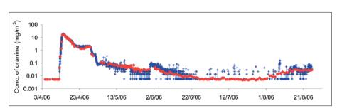
Fig. 4: Parallel measurements with field-fluorometer LLF-M (blue) and Luminiscence Spectrometer LS 30 (red) coincide well.
