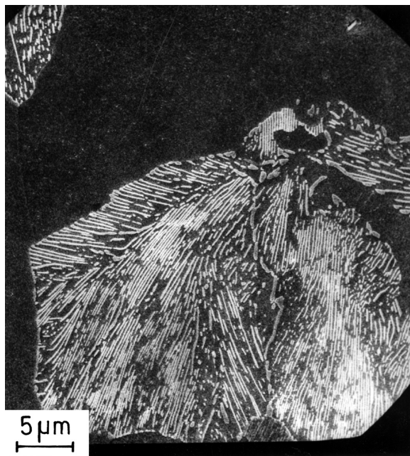
Fig. 11: Sword P 3621. SEM image of the ferrite pearlite microstructure.
