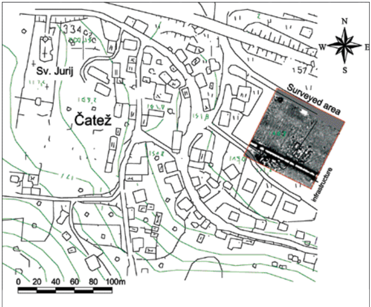
Fig. 34: Čatež along the Sava. Pedosequences on clays and loam. A diagram of the area investigated with a magnetogram of the vertical gradient of the magnetic field (Fluxgate gradiometer FM36).
