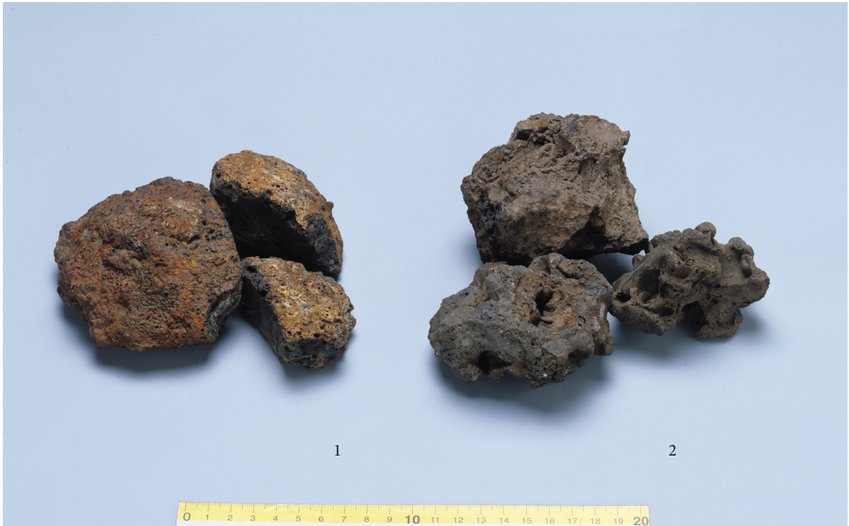
Fig. 4: Products of iron smelting – loaf-shaped iron blooms and pieces of iron slag. 1 the hillfort Grad by Šmihel, 2 Dunaj by Jereka (both from the collection of the National Museum of Slovenia). Photo T. Lauko.
