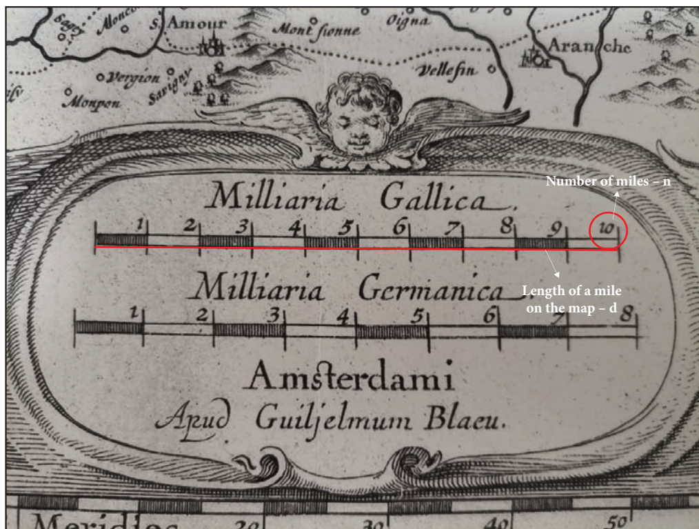
Figure 3: Display of the graphic scale on the map VZ VII, 50 with additional explanations of the graphic scale.
