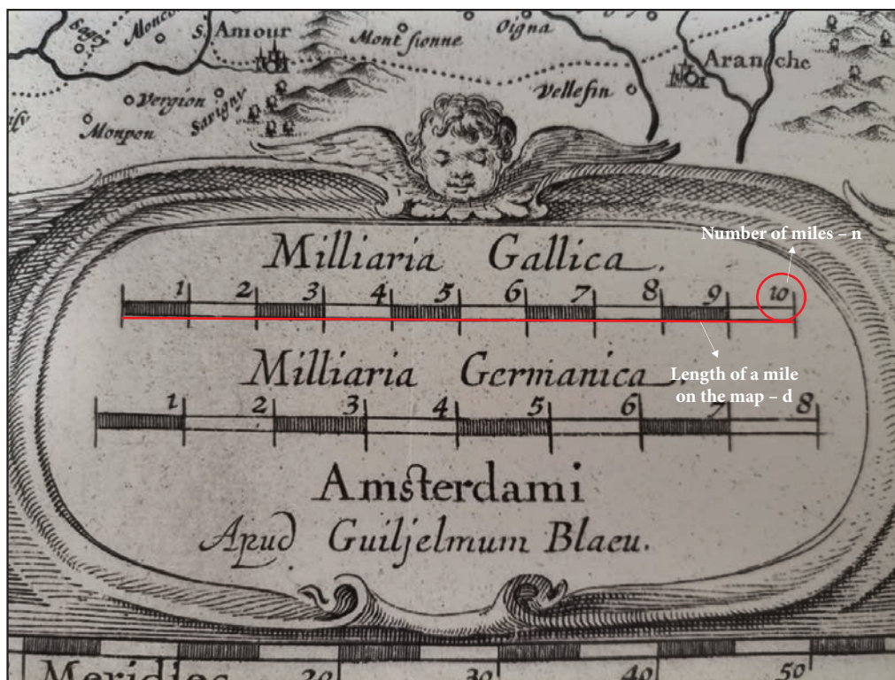
Figure 3: Display of the graphic scale on the map VZ VII, 50 with additional explanations of the graphic scale.
