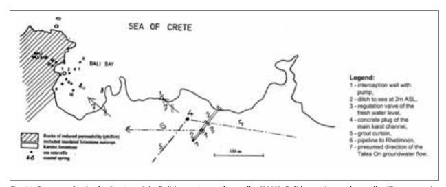
Fig. 14: Structures for the desalination of the Bali bay springs and estavelles (2008). Bali bay springs and estavelles (Economopoulos 1983).
