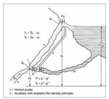
Fig. 4: Coastal spring of a conduit type (Kuščer 1950). Flow in a karst aquifer (Kuščer 1950).
