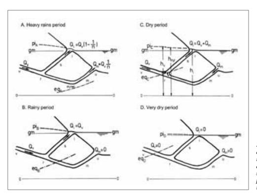
Fig. 7: Coastal spring with a siphon-like lower vein in a karst conduit flow aquifer, pi – piezometric surface, eq – equilibrium plane. Four Flow: Salinity regimes (Breznik 1989).
