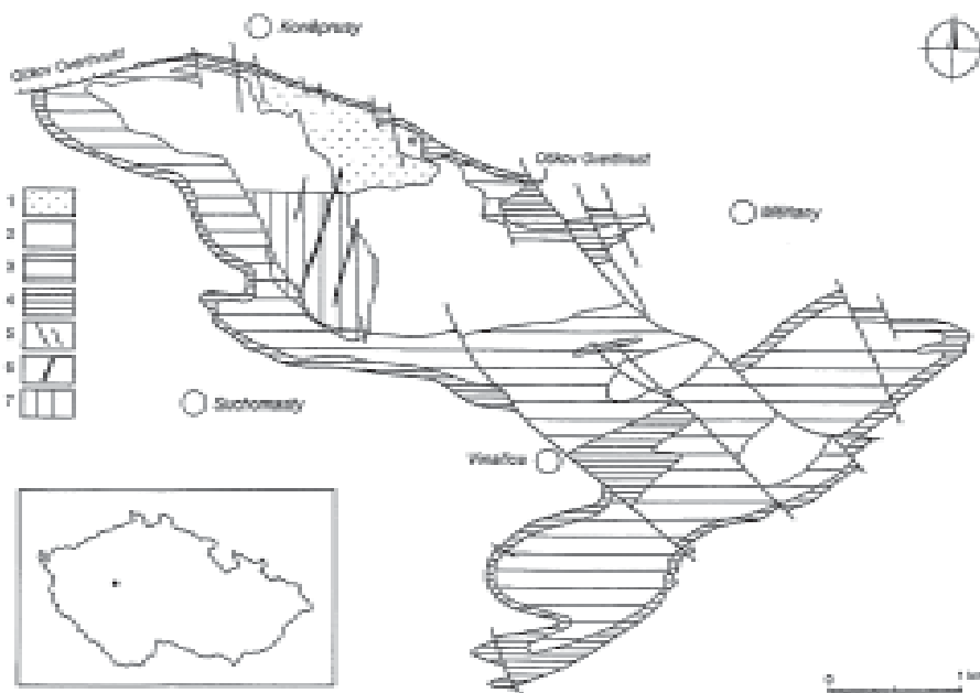
Fig. 4: Location of the Koněprusy site and simplified geological map (without Cenozoic cover; completed and modified after Klein et al. 1989)
